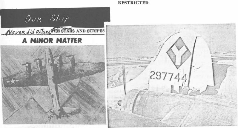
LITTLE THING like a smashed tail doesn't bother a Fortress, its B-17, on a mission over the Villaorba Airdrome in northstern Italy, was attacked by Nazi fighters using rocket shells. d although the tail section was almost completely shot away, p plane successfully returned to its base.
